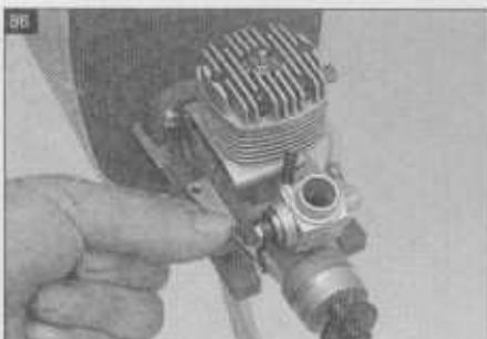
86 Attach the throttle rod to the arm of the carburetor.
