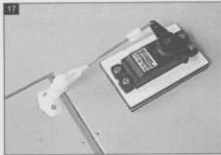
17 Attach the nylon clasp.
