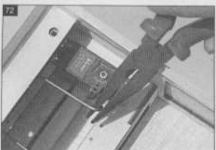
Bend "L" the elevator pushrod.
