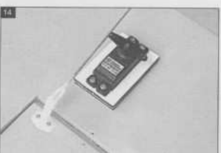
Attach the clevis to the control horn.
