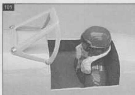
Install the canopy.
