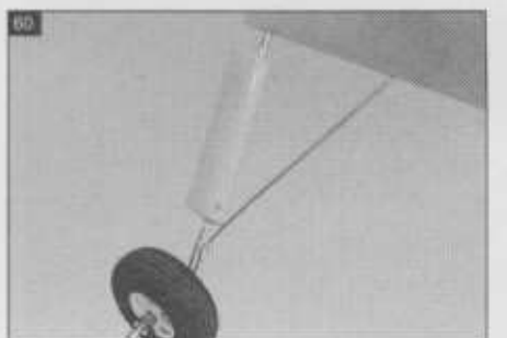
60 Attach the plastic cover for landing gear.
