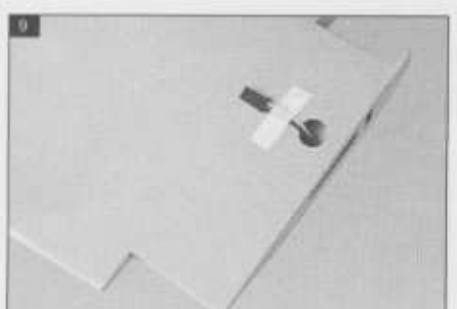
Using the masking tape, tape the servo lead onto the top of the wing.
