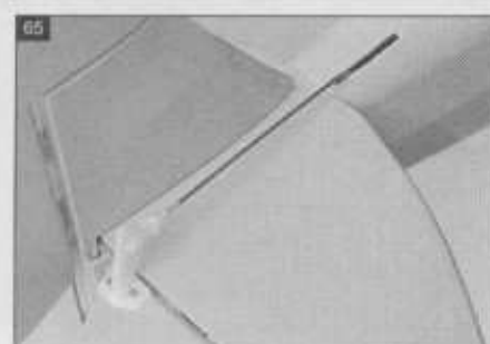
Attach the clevis to the control horn.
