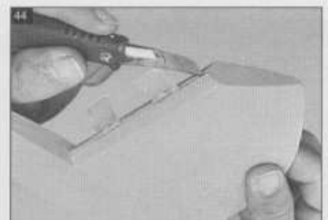
44 Make the slot for the tail gear.
