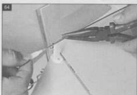
Slide the pushrod and attach the clevis to the elevator pushrod.
