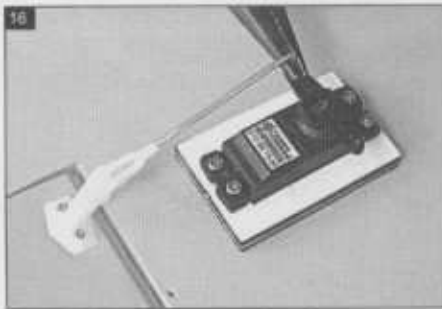
16 Bend "L" the aileron pushrod.
