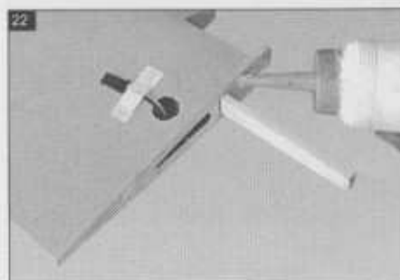
22 Apply the epoxy to the wing section.
